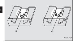
B- Fuse is OK C- Blown fuse
