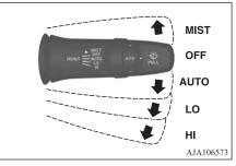
MIST- Misting function The wipers will operate once. OFF- Off AUTO- Auto-wiper control Rain sensor The wipers will automatically operate depending on the degree of wetness on the windscreen. LO- Slow HI- Fast
