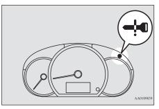
When the operation mode is in any mode other than OFF, if you try to lock the doors by pressing the driver's door lock/unlock switch, a warning lamp will blink and the outer buzzer will sounds for approximately 3 seconds and you cannot lock the doors.
