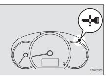
If the operation mode is in OFF and the driver's door is opened with the keyless operation key in the key slot, the warning lamp will blink and the outer buzzer sounds for approximately 3 seconds and the inner buzzer sounds for approximately 1 minute to remind you to remove the key.
