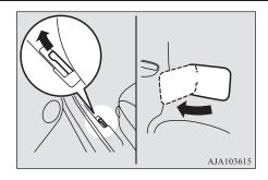
3. Open the fuel tank filler tube by slowly turning the cap anticlockwise.
