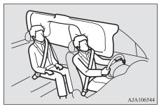
Deployment of side airbags and curtain airbags
