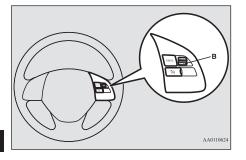
• When you release the SET - switch (B), the vehicle speed will be set.
