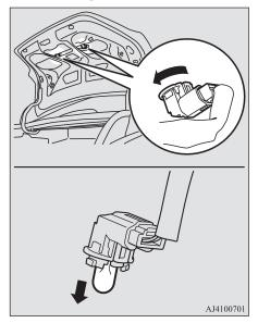
3. To install the bulb, perform the removal steps in reverse.
