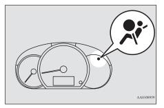
There is a supplemental restraint system ("SRS") warning lamp on the instrument panel. The system checks itself every time the ignition switch is turned to the "ON" position or the operation mode is put in ON. The SRS warning lamp will come on for several seconds and then go out. This in normal and means the system is working properly.
