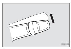
The wipers will operate once if the lever is moved to the "AUTO" position and the knob (C) is turned in the "+" direction when the ignition switch is in the "ON" position or the operation mode is in ON.
