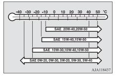
• Select engine oil of the proper SAE viscosity number according to the atmospheric temperature.
