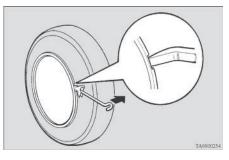
2. With the cover raised a little, pry it off completely using the jack bar. Insert the jack bar under the cover, and move it around the circumference, prying the cover away from the wheel little by little as you move the bar around.
