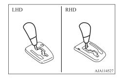
LHD (5 positions) LHD (6 positions) Ρ Ν D Ds D Ds RHD AJE101680 While depressing the brake pedal, Ø move the selector lever through the gate.
