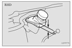
The fluid level is monitored by a float. When the fluid level falls below the "MIN" mark, the brake fluid warning lamp lights up. The fluid level falls slightly with wear of the brake pads, but this does not indicate any abnormality.
