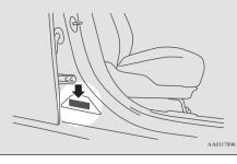
The plate shows vehicle identification number (1) and body colour code (2).
