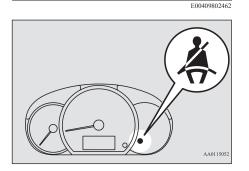
If the ignition switch is turned to the "ON" position or the operation mode is put in ON while the seat belt is not fastened, the warning lamp comes on and the tone sounds for about 6 seconds to remind the driver and the front passenger (if so equipped) to fasten the seat belt.
