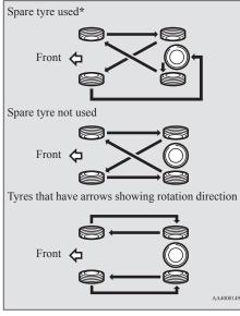
\*: If the spare tyre differs from the normal tyre, do not perform tyre rotation using a spare tyre.
