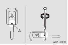
3. With the MITSUBISHI mark facing you, insert the cloth-covered tip of a straight blade (or minus) screwdriver into the notch in the remote control switch case and use it to open the case.
