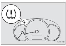
When the ignition switch is turned to the "ON" position, the tyre pressure monitoring system warning lamp normally illuminates and goes off a few seconds later.
