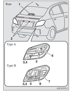
Type A: Bulb type stop and tail lamps Type B: LED type stop and tail lamps
