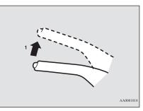
1- Firmly depress and hold the brake pedal, then pull the lever up without pushing the button at the end of hand grip.
