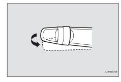
4. The headlamps will come on in the low beam setting for about 30 seconds. After the headlamps go off, the headlamps can be turned on again in the low beam setting for about 30 seconds by pulling the turnsignal lever towards you within 60 seconds of turning the ignition switch to the "LOCK" position or putting the operation mode in OFF.
