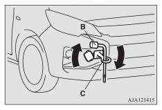
4. Secure the tow rope to the front towing hook.
